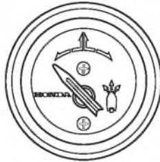
Rudder Meter [standard equipment (BFP60A LRTB type)] [optional equipment (other LRT and XRT types)]
