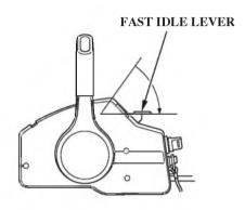
5. If the fast idle lever was used to start the engine, gradually lower the lever as the engine warms up.
