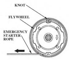
4. Set the knotted end of the emergency starter rope in the notch in the flywheel. Wind the rope clockwise around the flywheel, as shown.
