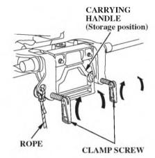
Attach the stern bracket to the boat transom by tightening the clamp screws. Push the carrying handle into the storage position. (tiller handle type)
