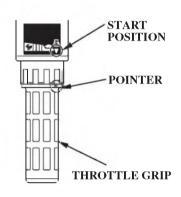
3. Align the engine start symbol "♂" on the tiller handle with the pointer "►" on the throttle grip.
