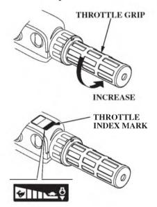
The throttle grip controls engine speed.
