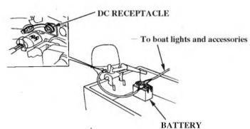
To prepare the outboard motor for connection to a battery, pull the cover off the DC receptacle, connect the battery charging wires to the plug. Attach the plug to the receptacle on the motor.
