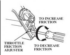
Adjust the throttle friction adjuster so the control lever will hold a constant throttle setting while cruising.
