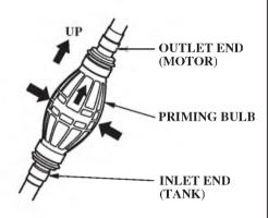
Hold the priming bulb with the outlet end higher than the inlet end. Squeeze the priming bulb several times, until it feels firm, indicating that fuel has reached the carburetor.
