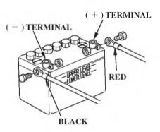
Honda BF25D and BF30D outboard motors produce a 12-volt, 4 or 10-ampere battery-charging current and are equipped for connection to a 12-volt battery. The battery-charging circuit is protected by a 15-ampere fuse located in the engine compartment.
