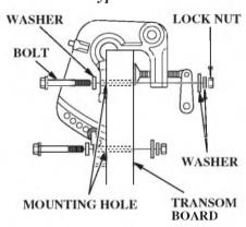
You may further secure the outboard motor by bolting the stern bracket to the boat transom. Use the optional mounting bolt and nut kit or other good quality stainless steel bolts, nuts, and washers. Apply silicone sealant to the bolt holes.
