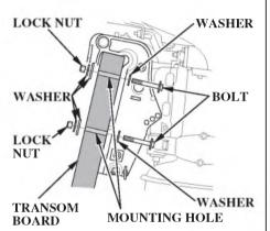
You may further secure the outboard motor by bolting the stern bracket to the boat transom. Use the mounting bolt and nut kit or other good quality stainless steel bolts, nuts, and washers. Apply silicone sealant to the bolt holes.
