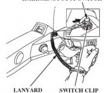
1. Put the emergency stop switch clip in the emergency stop switch, and attach the lanyard to your PFD (Personal Flotation Device) or to your wrist, as shown. The engine will not start or run, unless the clip is in the switch.
