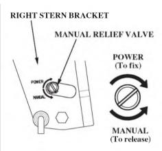
The outboard motor can also be tilted manually after opening the manual relief valve. This feature enables the outboard motor to be tilted when no battery is connected.
