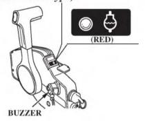
If the engine overheats, the red light will come on, and the engine protection system will limit engine speed.
