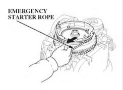
5. Pull the emergency starter rope slowly until resistance is felt, then pull briskly.
