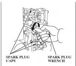
4. Inspect the spark plugs. Replace them if the electrodes are worn, or if the insulators are cracked or chipped.
