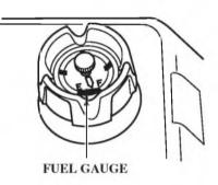
A fuel gauge is built into the cap of the portable fuel tank.
