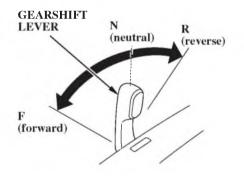
To shift gears, turn the throttle grip to the SLOW position, then move the gearshift lever to select F (forward), N (neutral) or R (reverse) gears.
