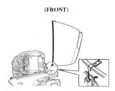
The engine cover latch fastens the engine cover to the outboard motor.
