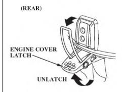
1. Unlatch and remove the engine cover.
