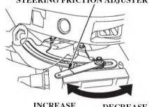
The steering friction adjuster adjusts steering resistance.
