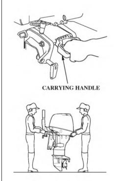
To carry, hold the outboard motor by the carrying handle, or hold by the carrying handle and the lug beneath engine cover lock lever, as shown.
