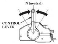
1. Move the throttle grip to the slowest speed and gearshift lever or control lever to N (neutral) position.
