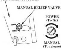
The outboard motor can be tilted manually after opening the manual relief valve. This feature enables the outboard motor to be tilted when no battery is connected.
