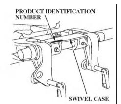
The product identification number is stamped on a plate attached on top of the swivel case.
