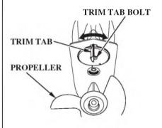
Adjust the trim tab with the engine stopped. Loosen the bolt above the trim tab, turn the trim tab, then tighten the bolt securely.
