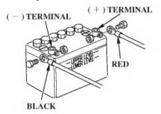
Connect the positive (+) battery cable to the positive (+) battery terminal, then connect the negative (-) battery cable to the negative (-) battery terminal.
