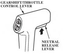
The control lever automatically locks itself in the N (neutral) position. To move the lever out of the N (neutral) position, you must squeeze the neutral release lever on the underside of the lever handle.
