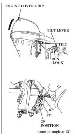
To tilt the outboard motor, move the tilt lever to the TILT position, then raise the outboard motor to the  $20^{\circ}$  or  $37^{\circ}$  position by pulling on the engine cover grip.
