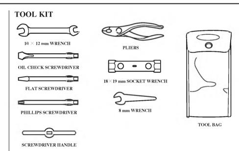
Individual items in the tool kit shown above can be purchased from an authorized Honda marine dealer and may be used for simple maintenance procedures and/or emergency repairs. Keep this tool kit or an equivalent onboard, so they will always be available if you need them.
