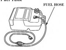
Empty the portable fuel tank into an approved gasoline container. Use a funnel to avoid spilling fuel. Rinse the fuel tank with nonflammable solvent to remove any accumulated sediment.
