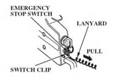
To stop the engine in an emergency, pull the clip out of the emergency stop switch by pulling the lanyard.
