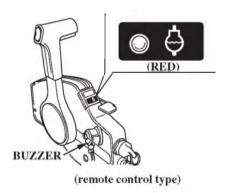
If the engine overheats, the red indicator light will come on, and the engine protection system will limit engine speed. If you are at cruising speed, engine speed will decrease gradually.
