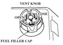
To refuel, turn the vent knob counterclockwise to the OPEN position, and unscrew the fuel filler cap.
