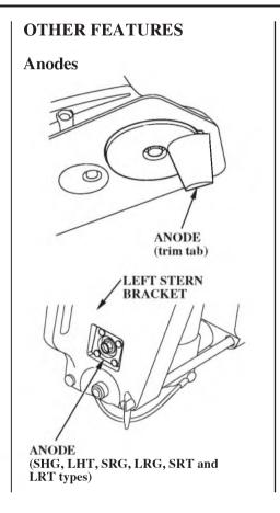
The anodes are made of a sacrificial material that helps to protect the outboard motor from corrosion.
