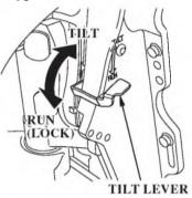
Moving the tilt lever to the TILT position allows the outboard motor to be tilted and moving the tilt lever to the RUN (LOCK) position locks the outboard motor in the desired position. Use the tilt lever to temporarily tilt the outboard motor when the boat is operating in shallow water, or mooring in shallow water. The tilt lever must be in the RUN (LOCK) position before operating the outboard motor or the motor could tilt up when operating in reverse.
