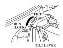
The tilt lever enables the outboard motor to be raised for shallow water operation, beaching, launching, or mooring.
