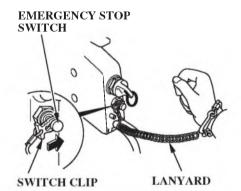
1. Put the emergency stop switch clip in the emergency stop switch, and attach the lanyard to your PFD (Personal Flotation Device) or to your wrist, as shown. The engine will not start or run, unless the clip is in the switch.
