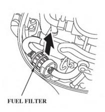
3. Raise the fuel filter, and remove it from the engine under case.
