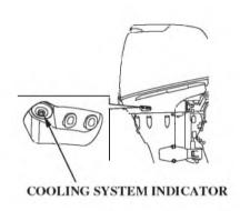
If overheating activates the engine protection system, idle the engine in neutral, and check the cooling system indicator.
