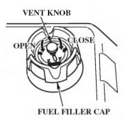
The cap is provided with a vent knob to seal the portable fuel tank for carrying it to and from the boat. Open the vent knob 2 or 3 turns before starting the engine.
